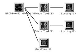
The new MPXbus tool (MPXbus Tool <2>) and the new Listing window (Listing<2>) will be created using default preferences. You will need to manually set the new preferences to reflect your target system. See "To Set the Inverse Assembler Preferences" on page 123 and "Setting the MPXbus tool preferences" on page 100.
