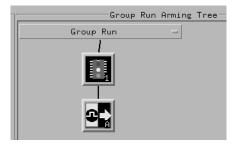
Selecting the **Group Run** button (at the very top of the Intermodule window or a logic analyzer window) will start the analyzer running. The analyzer will then wait for an arm signal. Now, when the emulation module transitions into "Monitor" from "Running" (or from "Reset"), it will send the arm signal to the analyzer. If the emulation module is "In Monitor" when you select **Group Run**, you will then have to go to the emulation module or your debugger interface and manually start it running.
