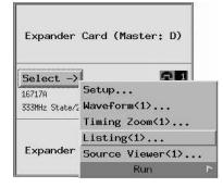
The logic analyzer will display the captured state data in the Listing display.
