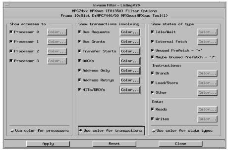
The inverse assembler filtering options allow you to display or hide certain types of microprocessor bus cycles. Because the filter options do not affect the data that is stored by the logic analyzer (they only affect whether that data is displayed), they let you display the same data in different ways.
